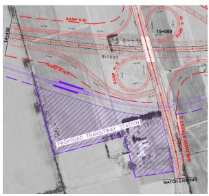
**Figure 33:** Excerpt of preliminary design drawing showing the proposed 407 Transitway station at Baldwin Street (Source: 407 East Individual Environmental Assessment and Preliminary Design Study, 2009, Appendix D–Recommended Design Plates)
