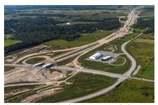
Figure 12: Highway 407, Phase 2 construction, looking southwest from the Bowmanville Avenue interchange (Source: Blackbird Infrastructure Group, August 2018)
