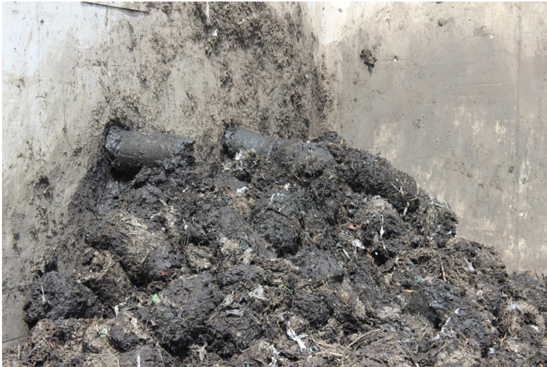
Figure 3-3-4 FITEC, Rothmuhle Biogas Plant: Extruded Solid Fraction from Biosqueeze Unit (to Composting)
