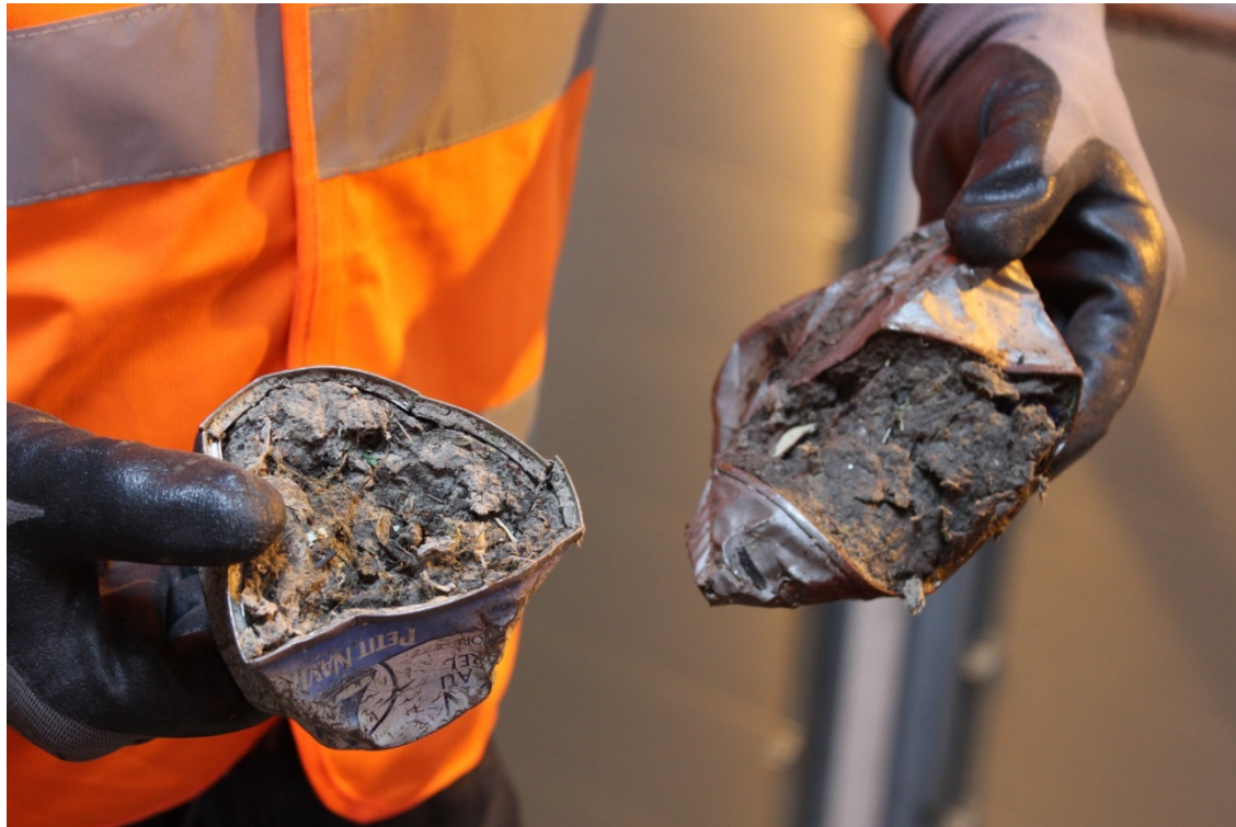
Figure 3-7-5 OWS Chagny AD Plant: Recovered Metal with Organic Content (output from commuting drum)
