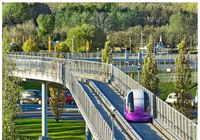
FIGURE 12. The Heathrow transport pod system provides a link from the T5 Business Car Park to the terminal and consists of 21 battery powered, driverless, zero emission vehicles (Golf Hotel Whiskey)
