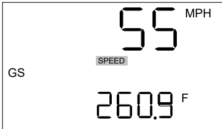
Figure 19. Sample Speed Measurement - Weather Filter ON
