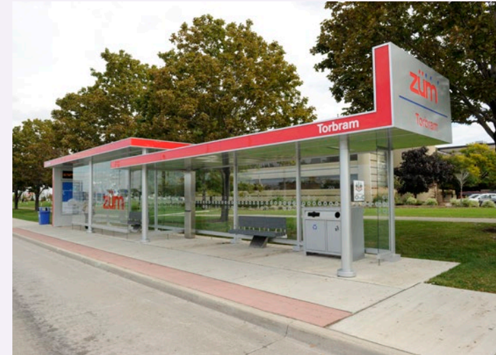
Figure 90. The design of this bus shelter along an arterial road establishes the stop as a prominent feature within the street while accommodating both interior and exterior waiting areas with seating and waste receptacles. Credit: Ministry of Transportation, Ontario.
