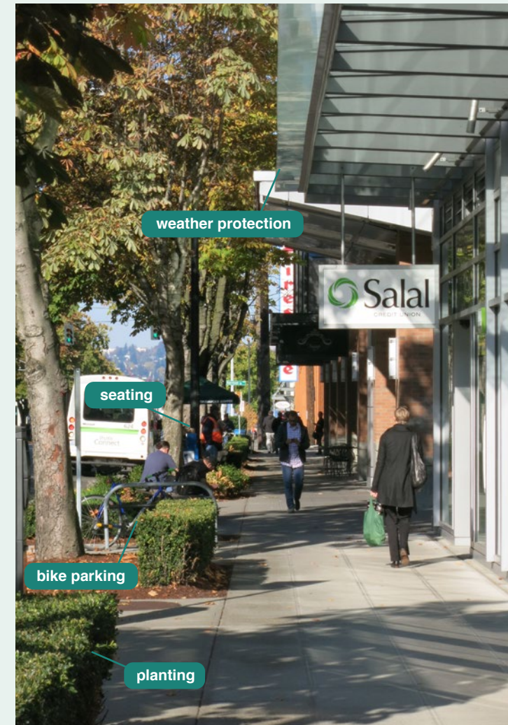
Figure 60. Canopies, generous landscaping, seating and bike parking contribute to user amenity alongside this bus stop.
