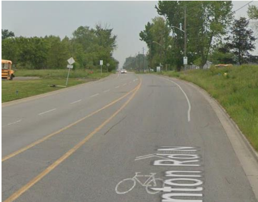
Picture 15. Sharrows Pavement Marking and Bike Route Begins Signage on Thornton Road N in Oshawa (Source: Google Streetview).
