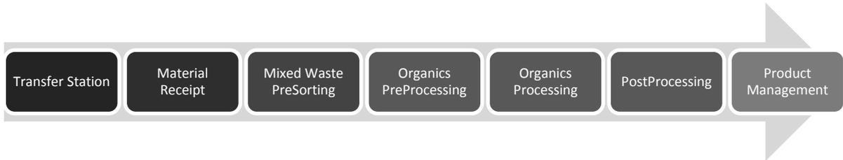
**Figure 5.1 Typical Mixed Waste Pre-Sort/Transfer and Organics Management Facility**
