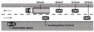
**Figure 5.4** The vehicle going 70 mph is the next strongest target going faster than the strongest.
