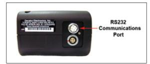
**Figure 6** Port location as shown on the SCOUT.
