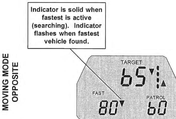
When operating the radar in Moving Opposite mode, the patrol vehicle and moving opposite road indicator will be on solid and the strongest vehicle speed will be displayed in the TARGET window.
