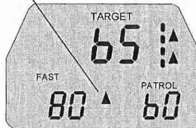
When operating the radar in Same-Direction mode, the same direction road indicator corresponding to the antenna selected will be on solid, and the strongest vehicle speed will be displayed in the TARGET window.
