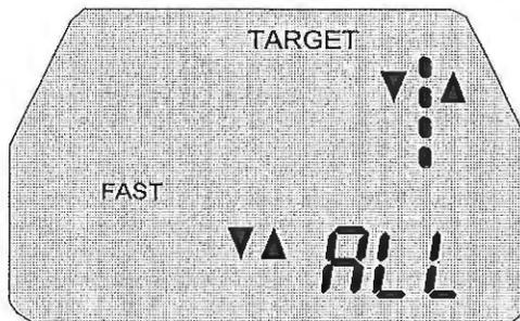
6. Momentarily press the AUD (audio) switch. The TARGET window will display "Aud" and a number from 1 to 5 indicating the audio level. With "Aud" displayed, press the RNG (range) switch until level 3 or 4 is displayed. Also, with "Aud" displayed, press the MODE switch, which will unquench the audio.
