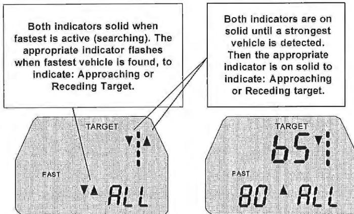
To monitor traffic in both directions (the Falcon HR will automatically indicate which direction the strongest and fastest vehicles are traveling), repeatedly depress the MODE switch until "ALL" is displayed in the PATROL window.
