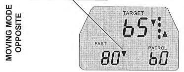
When operating the radar in Moving Opposite mode, the patrol vehicle and moving opposite road indicator will be on solid and the strongest vehicle speed will be displayed in the TARGET window.
