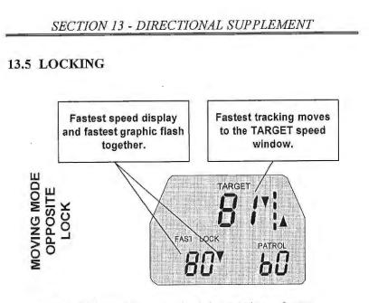
If the Lock button is pressed while tracking a fastest vehicle in any mode, the fastest speed will be locked in the LOCK window, and the fastest tracking will move to the TARGET window. After lock, both the LOCK window and the fastest indicator will flash together.
