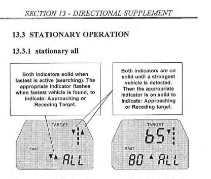
To monitor traffic in both directions (the Falcon HR will automatically indicate which direction the strongest and fastest vehicles are traveling), repeatedly depress the MODE switch until "ALL" is displayed in the PATROL window.
