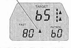
When operating the radar in Same-Direction mode, the same direction road indicator corresponding to the antenna selected will be on solid, and the strongest vehicle speed will be displayed in the TARGET window.
