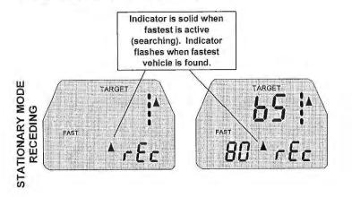
To place the unit in the stationary mode, monitoring receding traffic, repeatedly depress the MODE switch until "rEc" is displayed in the PATROL window.
