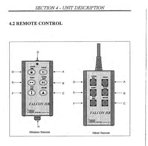
When the Falcon HR has a handle attached and is placed in the mount, certain functions can be controlled with the Wireless/Infrared (IR) remote. If the unit is attached to the optional pod, a wired or IR remote can be used.
