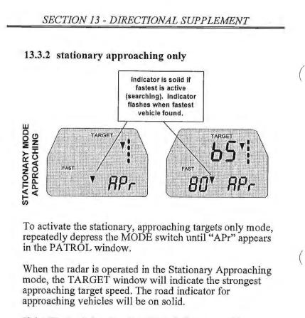
If the "Fastest" function is activated, the approaching fastest indicator will be on solid until a faster approaching vehicle is detected. At that time, the approaching fastest indicator will flash and the fastest speed will be displayed in the FAST window.
