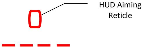
The LIDAR’s laser beam is invisible, but will be contained within the aiming reticle. This is your aim point for target vehicles.
