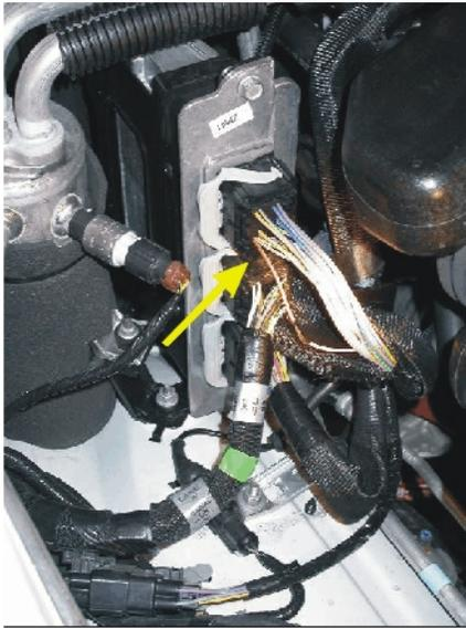
4. Using a scotch-lock t-tap and male quick-slide terminal, connect the red wire of the VSS cable to the vehicle OSS wire.
