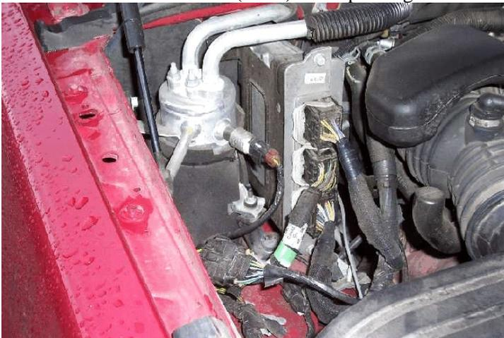
4. Using a scotch-lock t-tap and male quick-slide terminal, connect the red wire of the VSS cable to the violet/orange wire.
