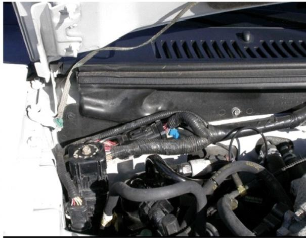
3. Using a scotch-lock t-tap and male quick-slide terminal, connect the red wire of the VSS cable to the vehicle VSS wire.
