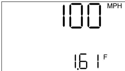
The number at the top is the model number of the instrument. The number at the bottom is the revision level of the instrument's internal software. MPH and F indicate the factory default speed and range units in effect at the time the instrument was shipped.
